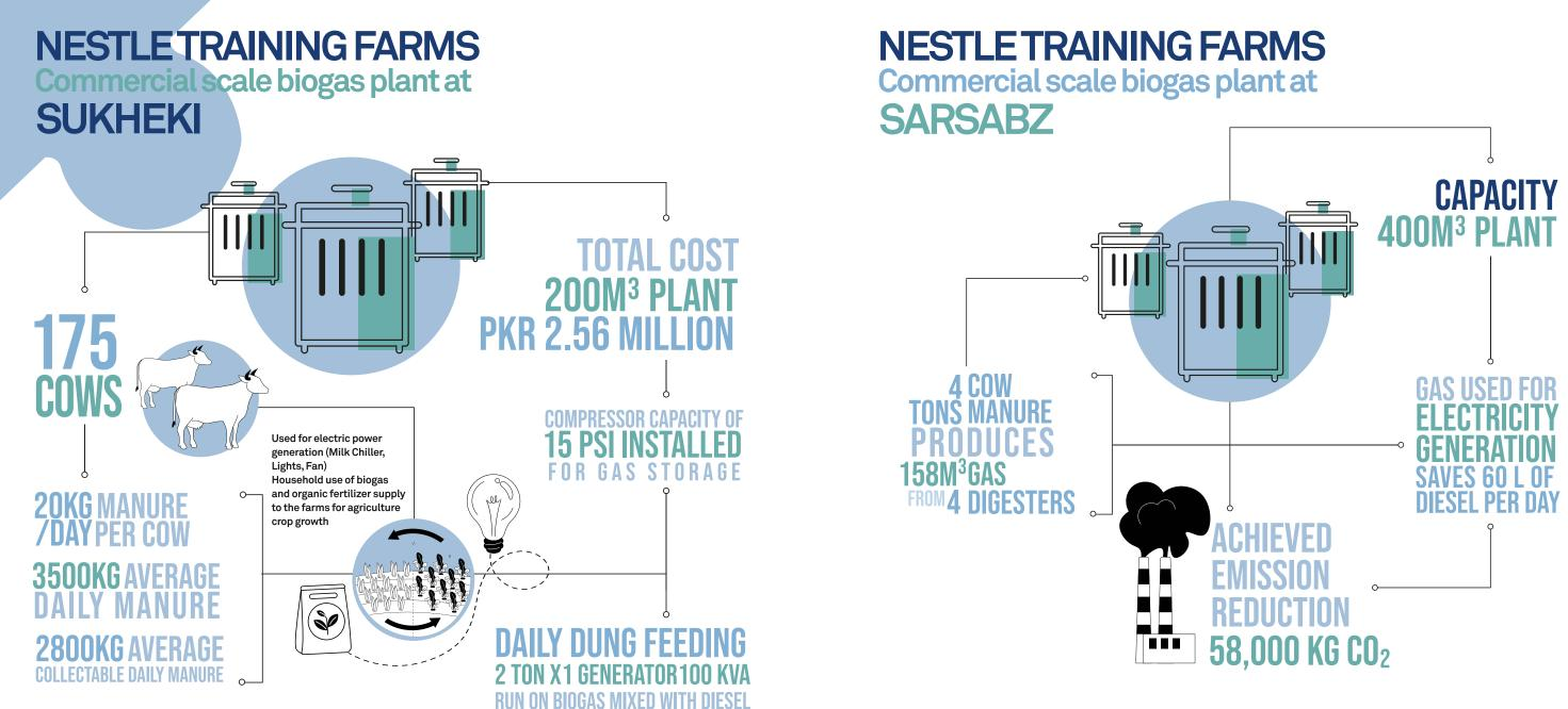
Nestle Pakistan installed another biogas plant of 400m3 capacity at Sarsabz farm 2014, this time, without the assistance of Winrock International, proving that such multi-stakeholder biogas projects have the power to achieve sustainable uptake and scaleup of biogas plants.
